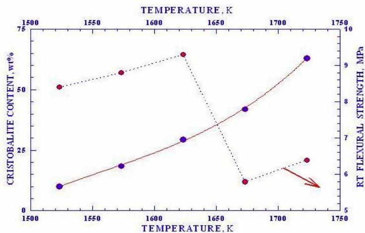
Fig.12: Variation of flexural strength with cristobalite content
