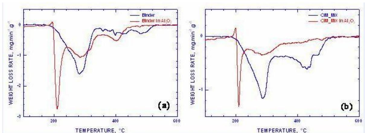
Fig.9 Thermal degradation behavior of binder through TGA
