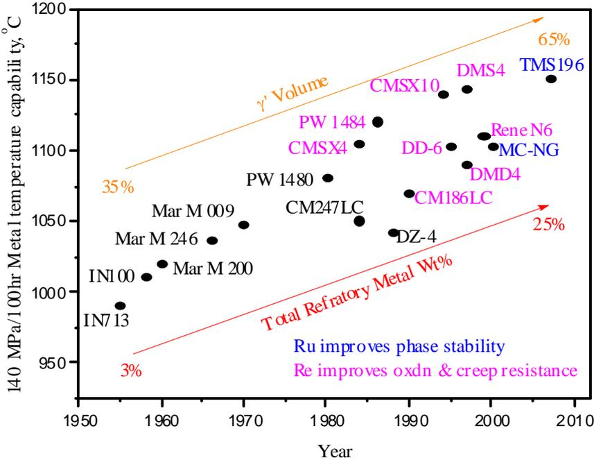
Fig. 4: Chronological development of cast Ni-base superalloys
