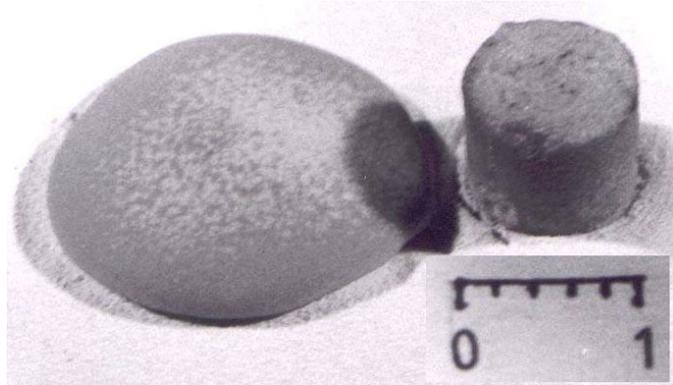
Fig.8 Shape distortion and collapse of CIM part during de-binder
