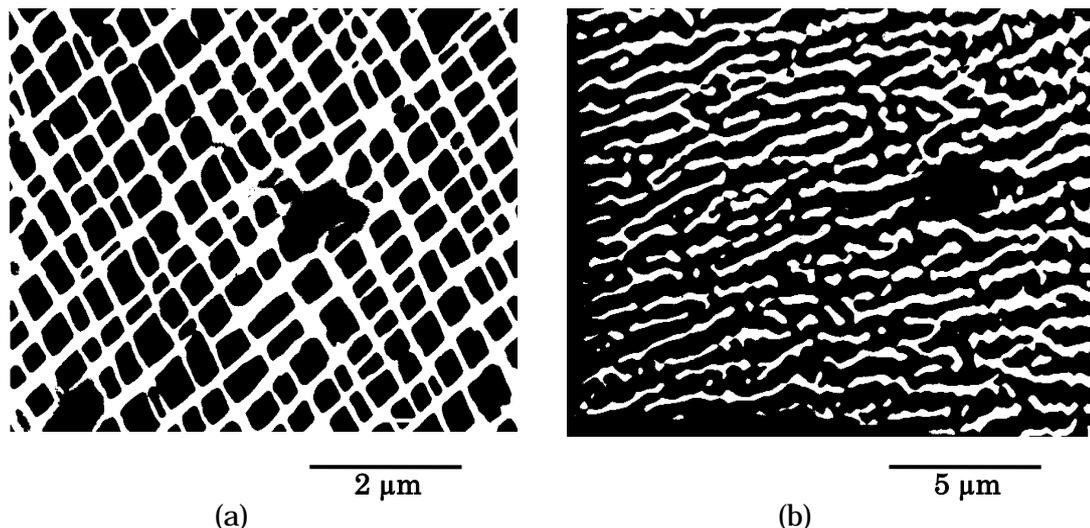
Fig. 3 (a): Cubic  $\gamma'$  precipitates of superalloy DMD4, aged at 1150°C after solution treated at 1330°C; (b): Rafted  $\gamma'$  structure in creep ruptured superalloy DMD4.
