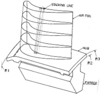
Fig. 6 Definition of Aerofoil Geometry
