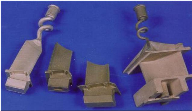
Fig. 14: (a) Hollow DS blades in alloy DMD4. (b) Single Crystal blades in alloy DMS4.
