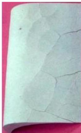
Fig.11: Sintering crack on core
