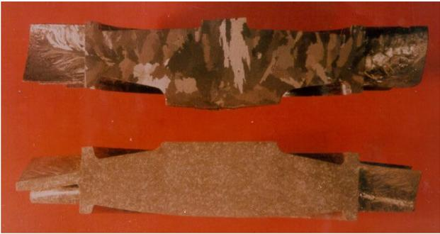
(b) Coarse grain conventional casting (above)
