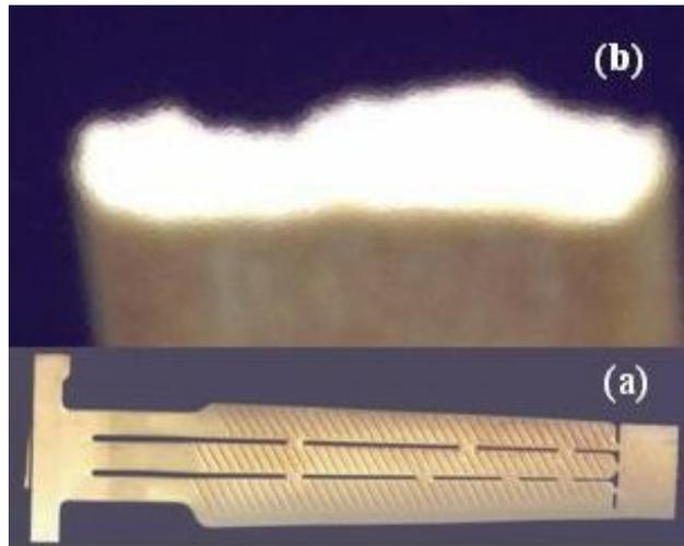
Fig.10 (a) LPT blade green core thermally degraded at 210°C. (b) Its cross-section
